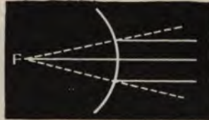
FIG. 142.—Reflection by a Convex Mirror.
